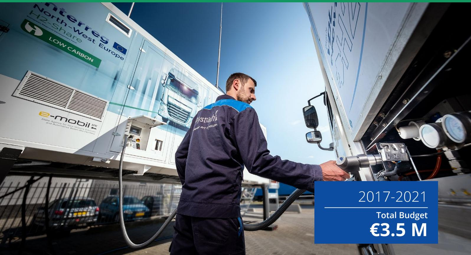
Refuelling the hydrogen truck at the mobile refueler during the first demo at Breytner in the Netherlands
