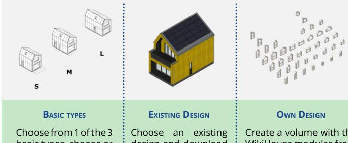
basic types, choose or design your own floor plan, then determine facade openings and finishes. Choose an existing design and download the corresponding files and find out what modifications, if any, are needed. Create a volume with the WikiHouse modules from the toolbox and situate the design on the site. Position the windows to suit the layout of the design and choose finishes as desired.
